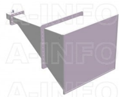
LB-340-20-C-NFSPO Standard Gain Horn Antenna 2.2-3.3GHz 20dB Gain N Type Female
