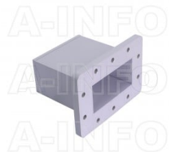
340WECAS Endlaunch Rectangular Waveguide to Coaxial Adapter 2.2-3.3GHz WR340 to SMA Female
