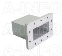
340WECAN Endlaunch Rectangular Waveguide to Coaxial Adapter 2.2-3.3GHz WR340 to N Type Female
